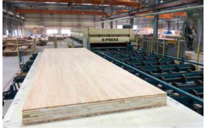
18. Hinoki CLT motherboard (3 m × 12 m)
