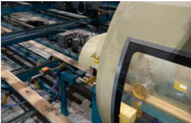
13. Finishing planing of lamina (thickness 30 mm)
