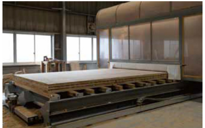
20. Cutting and machining with dedicated CLT processing equipment
