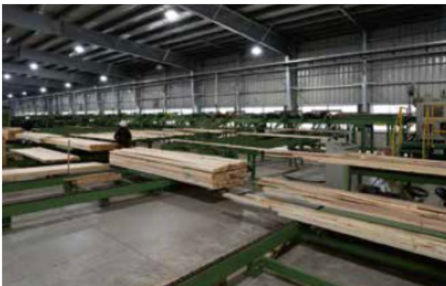
9. Young's modulus measurement and sorting of lamina (all pieces)
