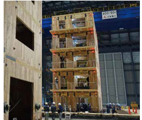
In 2015, a shaking table experiment was conducted at the National Research Institute for Earth Science and Disaster Resilience (NIED) on the 3D shaking table “E-Defense,” using five-story and three-story buildings. Input motions larger than those observed during the Great Hanshin-Awaji Earthquake were applied to examine deformation and damage, confirming that the buildings did not collapse.
