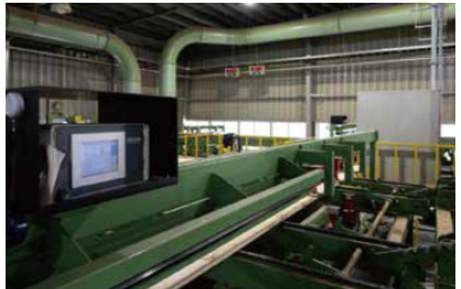
8. Moisture content measurement of lamina (all pieces)
