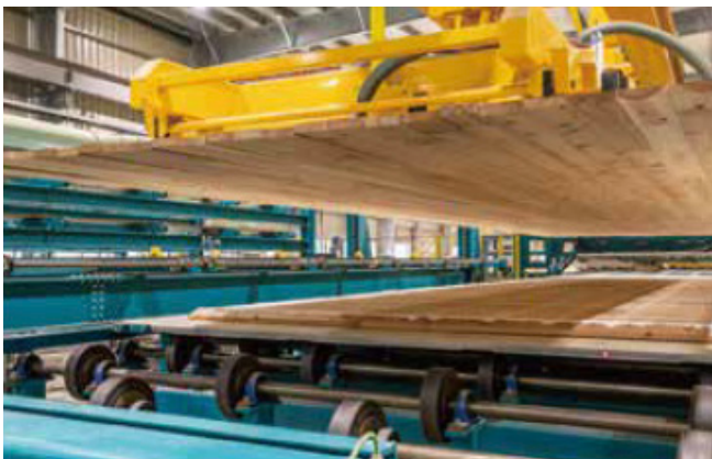
15. Lamination of lamina (3, 5, 7, or 9 layers) into CLT panels
