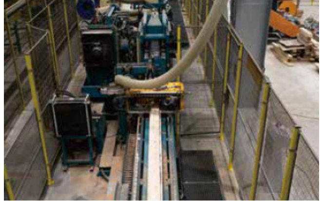
12. Longitudinal joining of lamina (finger joint)
