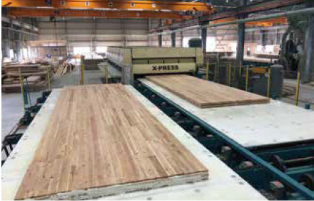
17. Sugi CLT motherboard (3 m × 12 m)
