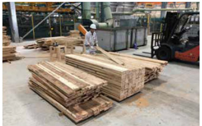
10. Visual grading of lamina [optional process]
