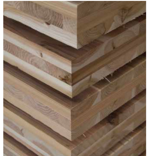
3-ply Sugi CLT, 90 mm thick
