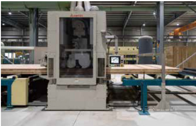
19. Sanding finish of CLT surface [optional process]
