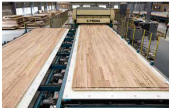
16. Pressing CLT (adhesive curing)
