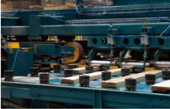
11. Finger-joint processing of lamina ends
