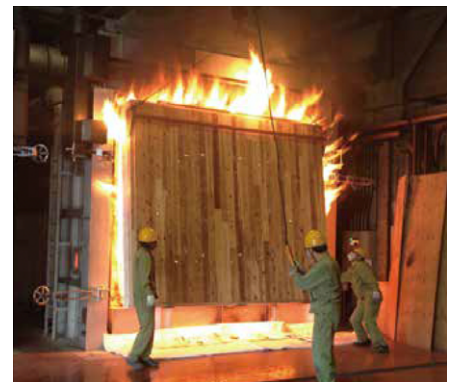
A fire resistance test of CLT exposed walls in quasi-fire-resistant construction was conducted at the fire testing furnace of the Japan Housing and Wood Technology Center. Utilizing the property of wood that chars inward at a slow rate of approximately 1 mm per minute, it was confirmed that a 90 mm thick CLT wall could resist burn-through for more than one hour.
