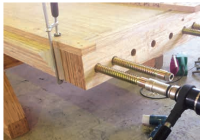
Embedding of Lag Screw Bolt LSB
